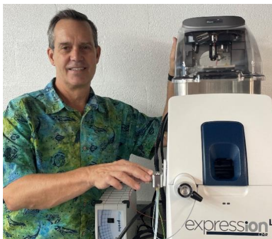
Gary Van Berkel standing next to a Van Berkel Ventures, LLC mass spectrometer fitted with both an Advion Touch Express Open Port Sampling Interface (right hand, front) and a Prosolia flowprobe (left hand, top back). Both commercial products are based on his inventions
